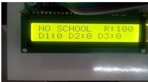
Fig 11: Indication of speed of DC motor when vehicle is far away from school zone
