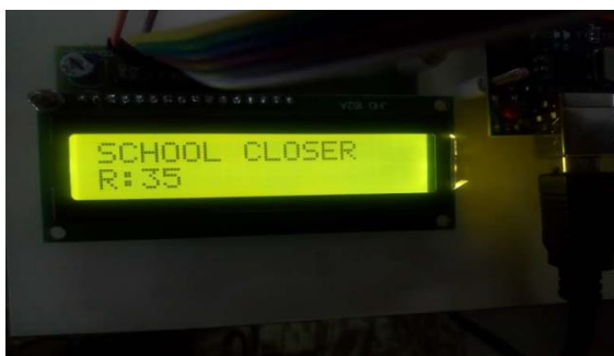
Fig 12: Indication of speed of DC motor when vehicle is closer to school zone
