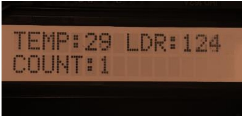
Figure 2 LED display showing the activities and parameters of the atmosphere
