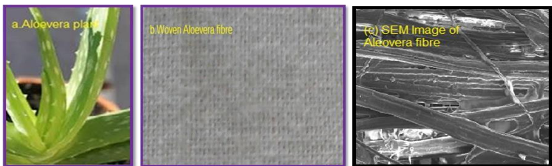
a) Aloe vera plant (b) woven Aloe vera fibre (120 GSM) (c) Microscopic image of Aloe vera (diameter-0.3 mm)
