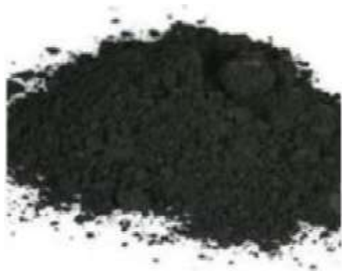
FIG.1 ACTIVATED CARBON POWDER(GROUNDNUT SHELL+COCONUT SHELL
