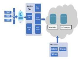
The layered architecture of CAGS ensures communication between the components. The presentation tier has the user interface to get input and deliverdesired output to the person in user understandable format. Service tier takes the input from the user, makes logicaldecisions and executes the processes.
